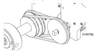
10. Align pulleys as shown below and tighten screws.
