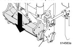
5. Slide single pulley over long axle.
