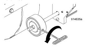
Install two angular inserts on bead dispenser and tighten screws.
