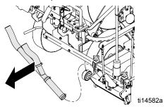
Loosen screw and remove bead dispenser engagement wheel.
