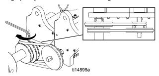
11. Attach pulley guard and tighten two screws.
