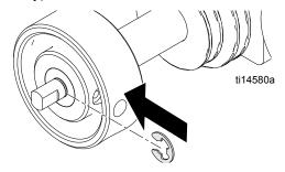
8. Slide pulley onto short axle.
