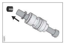
While holding the pump body upside down start threading the new packing assembly in by hand.
